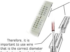
Under the plastic cover, the breadboard has metal rails under each connected row. Wire placed into the holes is connected to adjacent holes as the rails "pinch" a physical connection.
