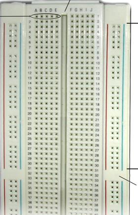
Longitudinal connections (usually for power.) All 25 sockets along the green line in this example are connected. So are the 25 sockets along the red line.
