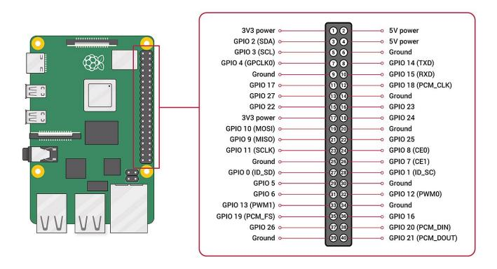
Raspberry Pi GPIO Pins: Any of the GPIO pins can be designated (in software) as an input or output pin and used for a wide range of purposes.
