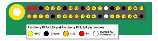
Note: the numbering of the GPIO pins is not in numerical order; GPIO pins 0 and 1 are present on the board (physical pins 27 and 28) but are reserved for advanced use (see below).
