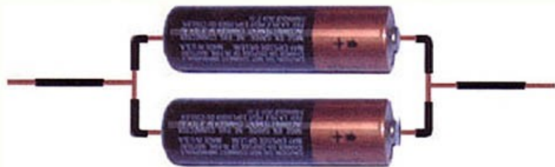
Batteries in parallel.
