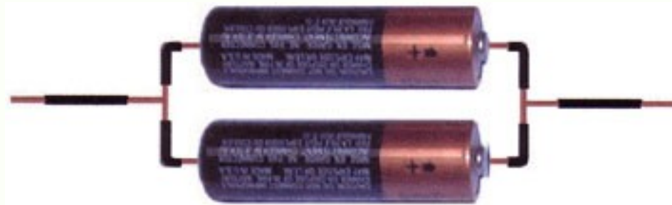
Batteries in parallel.
